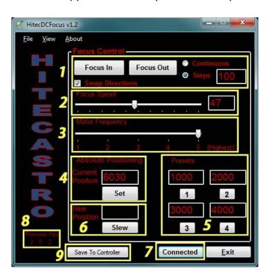
Once you have your power, motor, and USB cable plugged in click the 'Connect' (7) Button. If all is well, the text of the button will change to 'Connected' and the focuser will retrieve the current settings from the unit.
