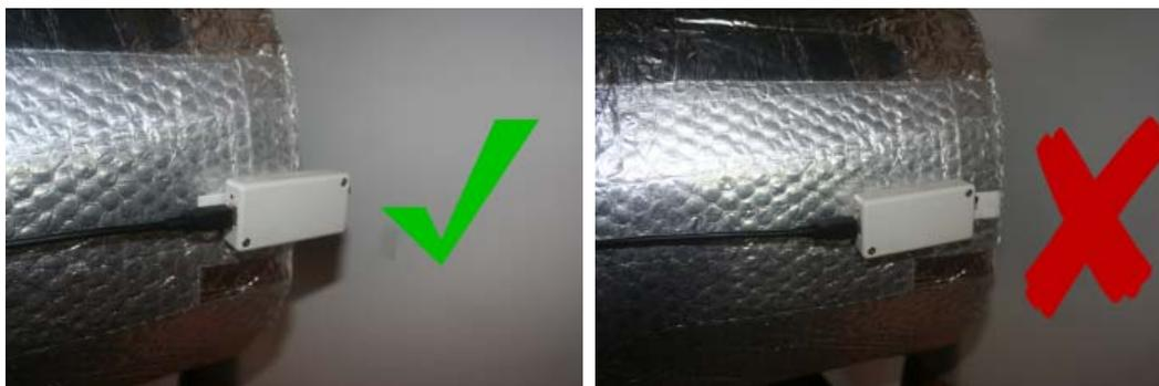
Note the incorrect position allows the dewshield to partially obstruct the field of view of the sensor. In short if you ensure that the sensors slightly protrude the front of your telescope/dewshield you have mounted the device correctly.
